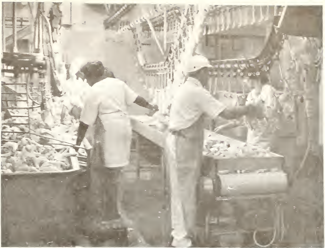
Figure 5.--Undergrade birds collected on the belt conveyor are transferred to overhead conveyors (cut-up line).
